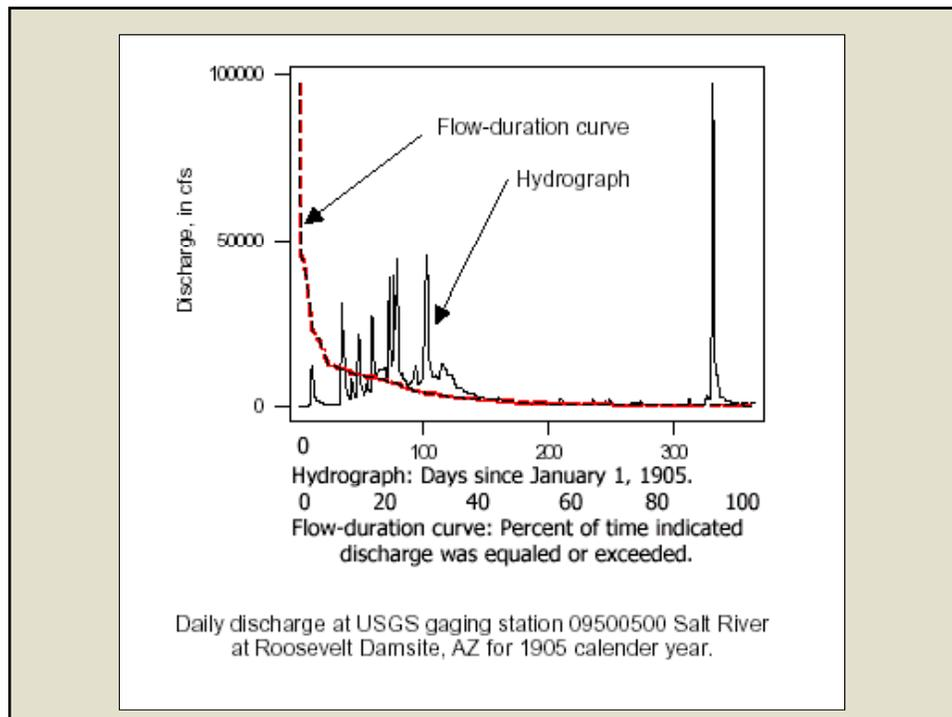
The flow-duration curve is a cumulative frequency curve that shows the percent of time specified discharges were equaled or exceeded during a given period.
