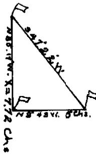
To determine the distance across the river I set a flag on line on a sand bar across the channel for triangulation point. Then from the triangulation point on the East side of the Verde River channel, I measure a base N. 9° 43' W., 5.00 chs., from which the flag on West bank of channel bears S. 47° 22' W. Therefore, the distance is the tan. 57° 8' x base or  $1.5447 \times 5.00$  equal 7.72. 2.50 + 7.72 makes
