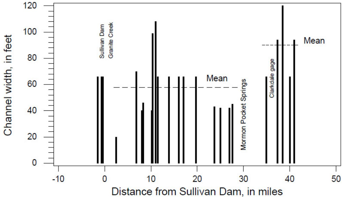
Surveyed channel widths of the original land surveys are considerably greater than measured widths.
