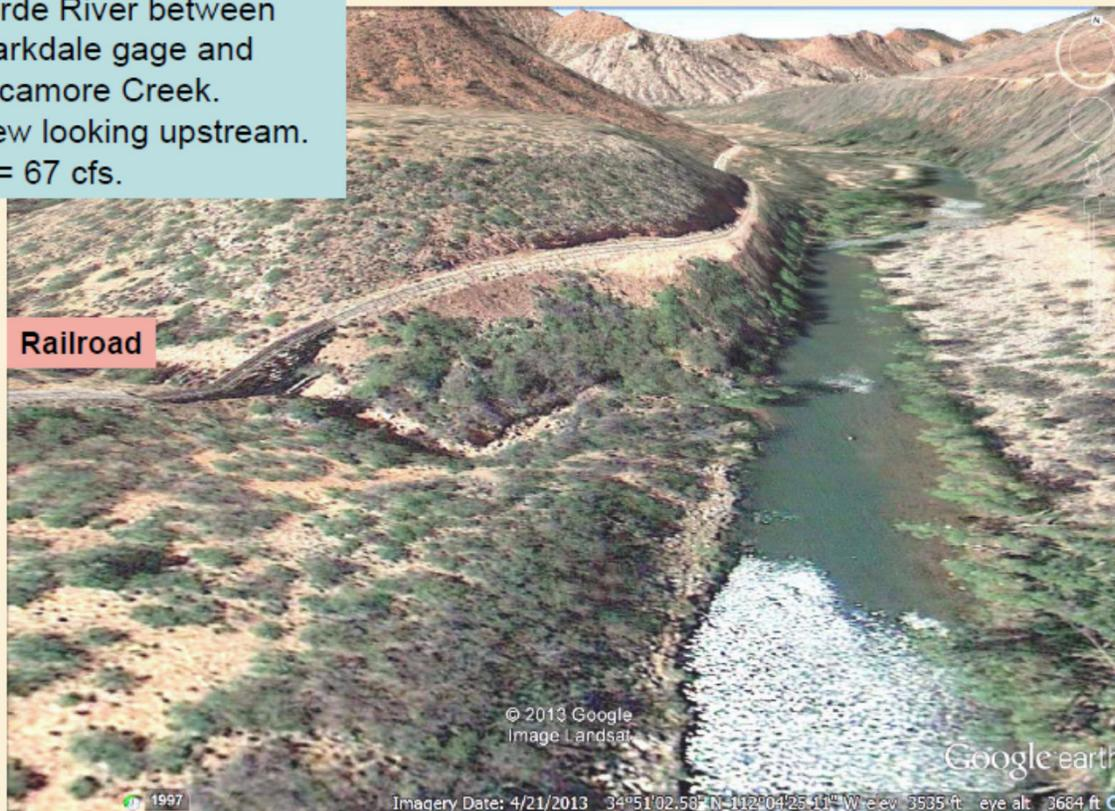
Large debris (boulders) from side slopes. Obviously only very large high (kinetic) energy flow will move such large obstructions. Also, energy is lost (with a corresponding decrease of velocity and increase in depth) as streamflow encounters this rough channel material.
